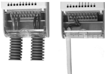
SSW60 is provided with two quick terminal covers with strain relief on both sides. If a flexible hose is required to be connected on the primary side, the enclosed extra cover is used. Flexible hose is suitably used in installations where single-insulated cables are connected, and strain relief is used when double-insulated cable is connected to the LED controller.
